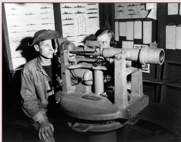
Base end station with a depression position finder scope (courtesy of John Martini, http://cdsg.org/old/ )
